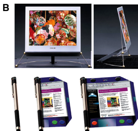
(B) Organic light emitting diodes can be used to make thin and flexible displays. Adapted by permission from Nature, Forrest [2].
