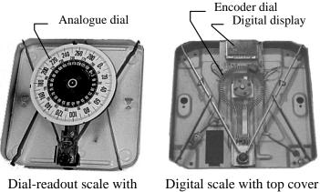
Dial-readout scale with top cover removed (Note analogue indicator wheel)
