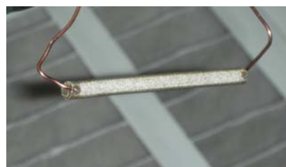
Air Sample Collection Tube (MS/GC)
