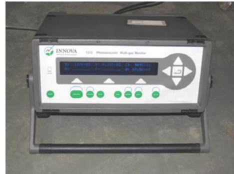
Direct Read Innova Instrument Used
