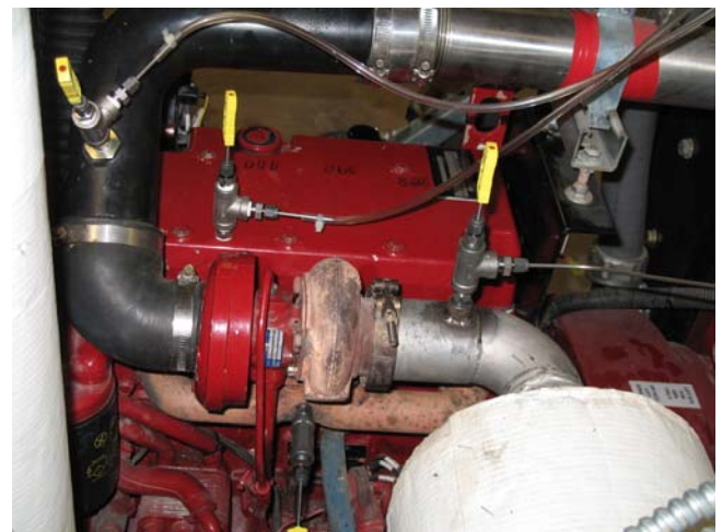
Figure 8. Turbocharger Instrumentation Setup
