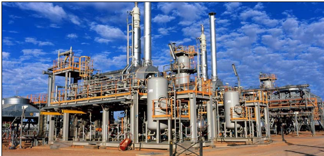
Figure 13. An Amine-Based CO 2 Capture System Used to Purify Natural Gas at BP's In Salah Plant in Algeria
