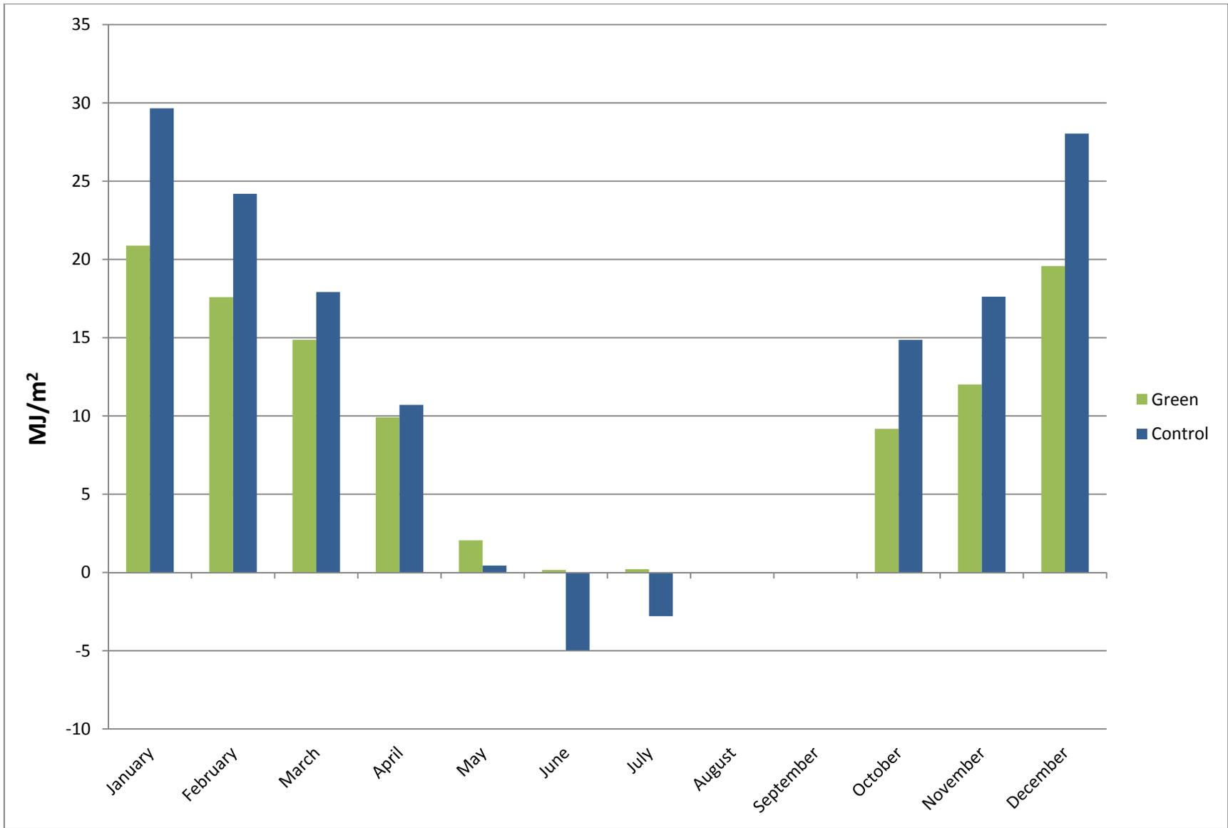
**Figure 5:** Heat loss or gain per month for Hamerschlag Hall green roof and Porter Hall control roof in 2009
