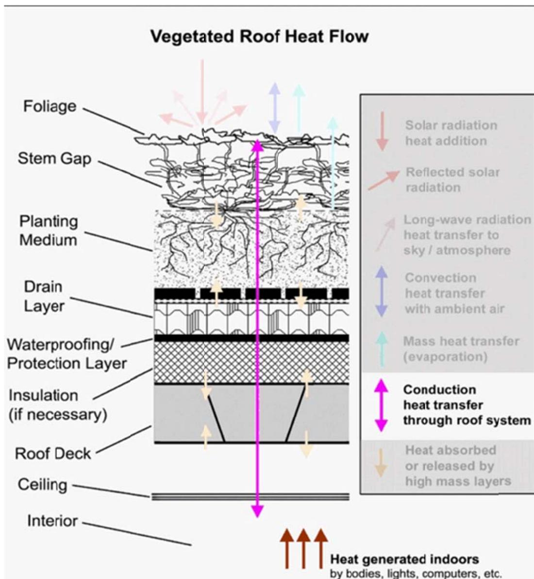
**Figure 1:** Modes of Heat Transfer Through Generic Green Roof. Source: Wark (2010)
