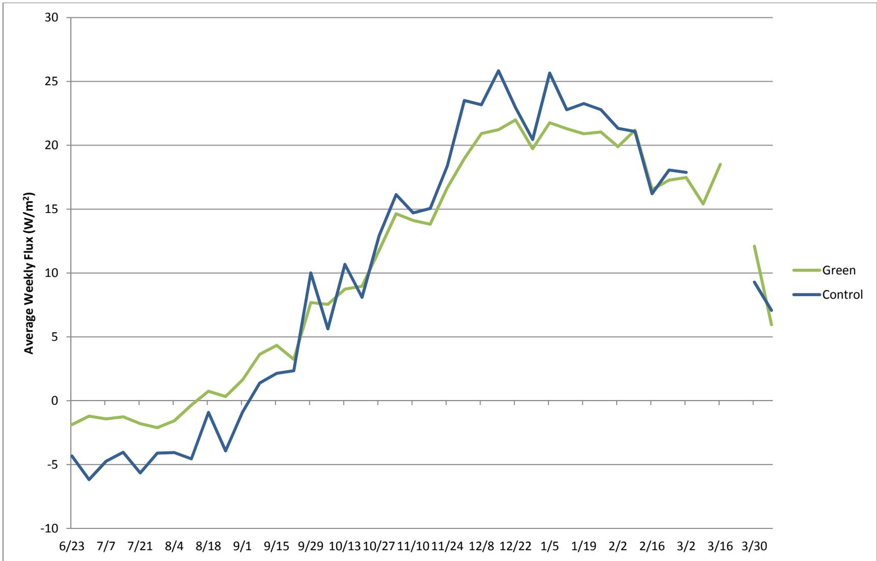
**Figure 7:** Average weekly heat flux through conventional roof layers in green roof and control roof at ACOB, June 2010 through April 2011
