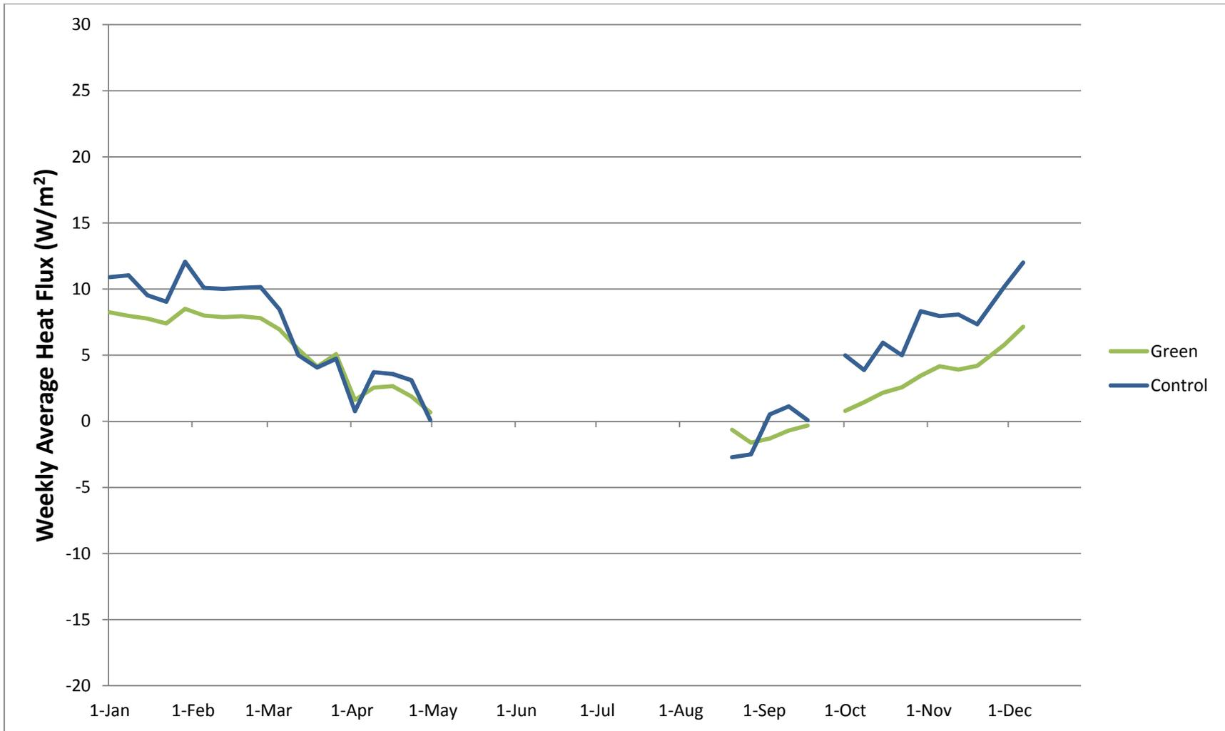
**Figure 4:** Average weekly heat flux through conventional roof layers in Hamerschlag Hall green roof and Porter Hall control roof in 2010
