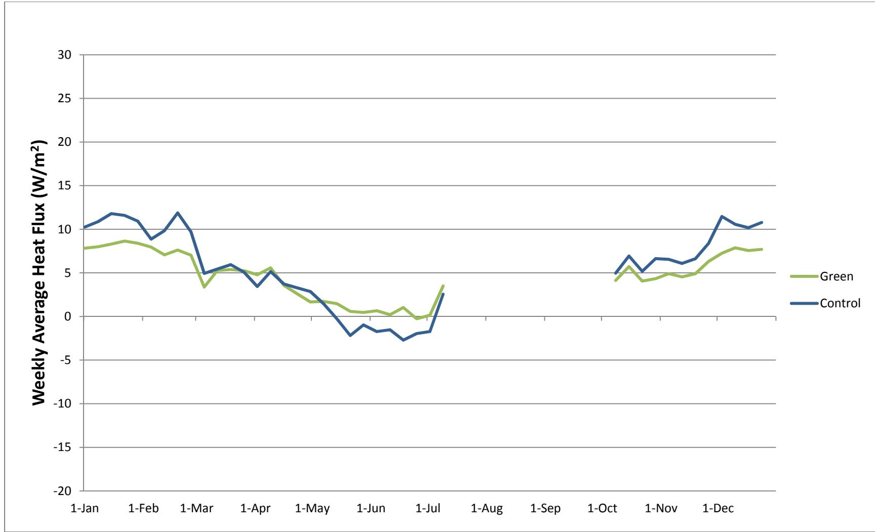
**Figure 3:** Average weekly heat flux through conventional roof layers in Hamerschlag Hall green roof and Porter Hall control roof in 2009
