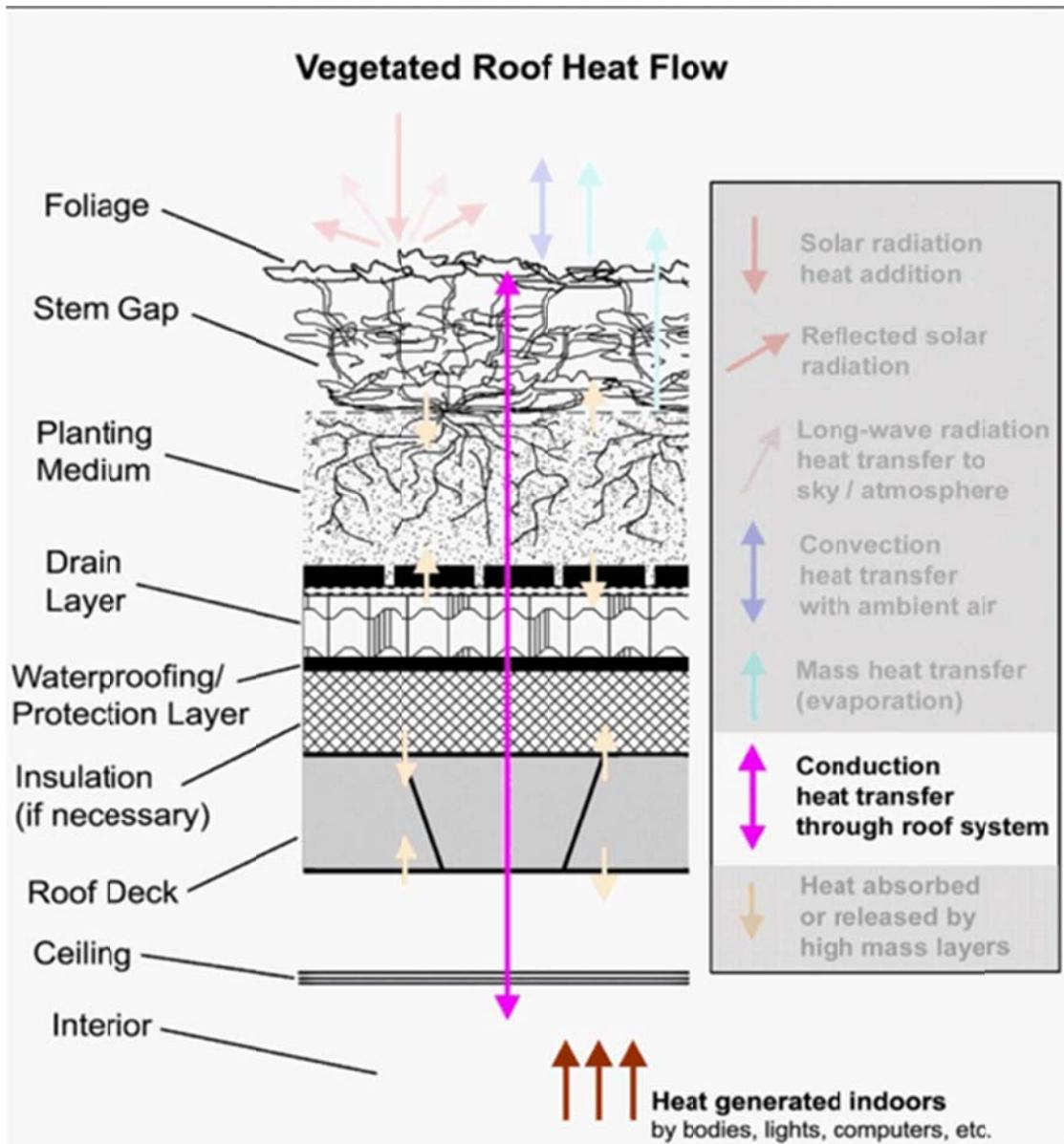
**Figure 1:** Modes of Heat Transfer Through Generic Green Roof. Source: Wark (2010)
