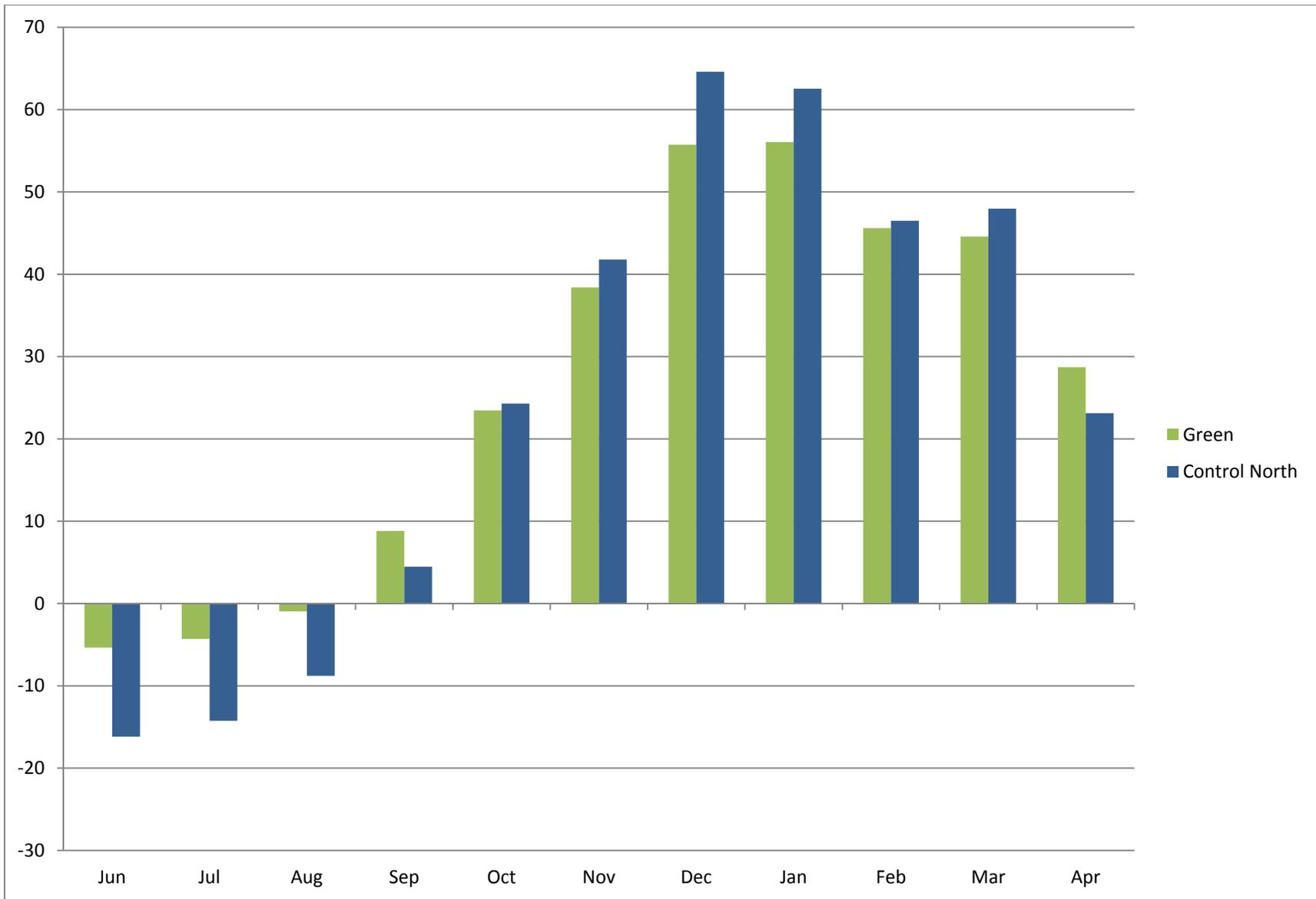
**Figure 8:** Heat loss or gain per month for ACOB green roof and control roof, June 2010 through April 2011
