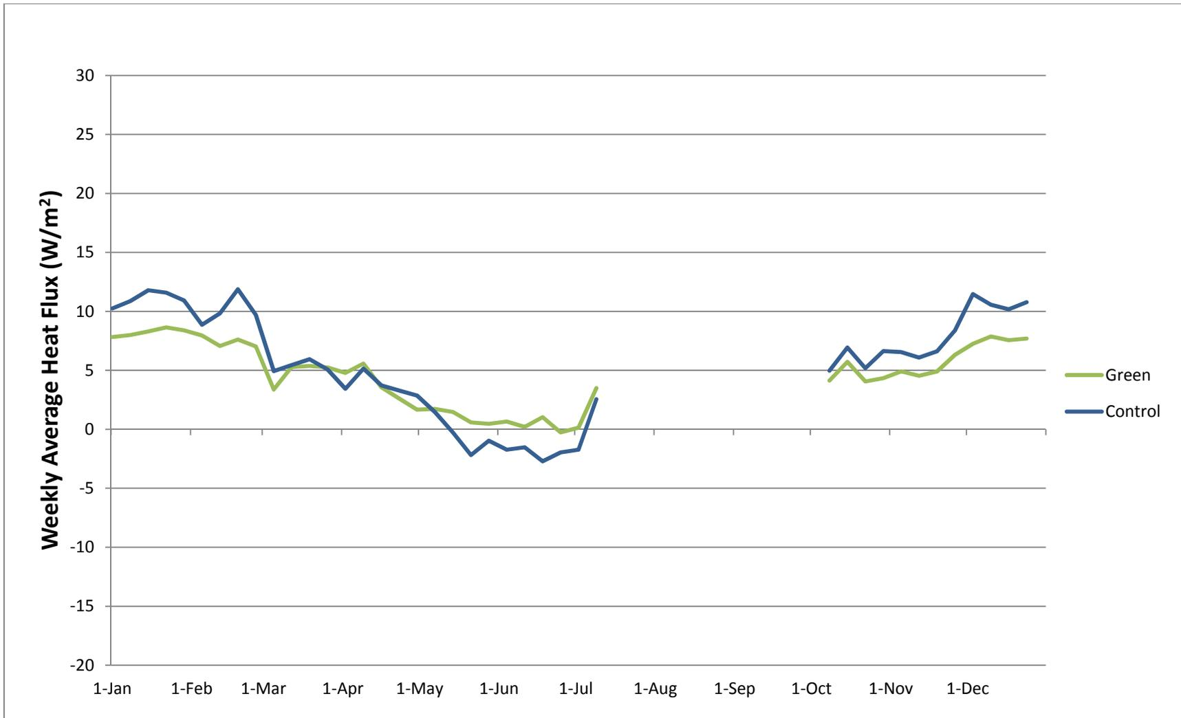
**Figure 3:** Average weekly heat flux through conventional roof layers in Hamerschlag Hall green roof and Porter Hall control roof in
