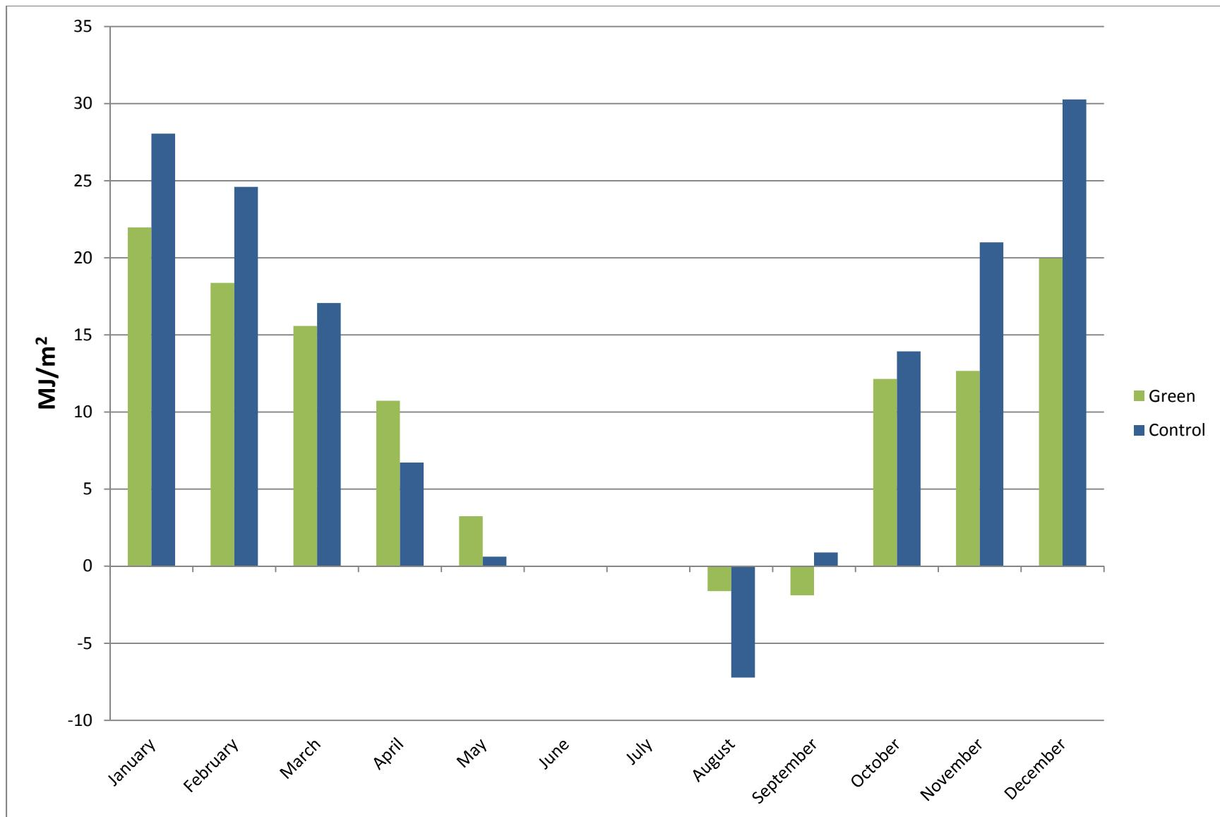
**Figure 6:** Heat loss or gain per month for Hamerschlag Hall green roof and Porter Hall control roof in 2010
