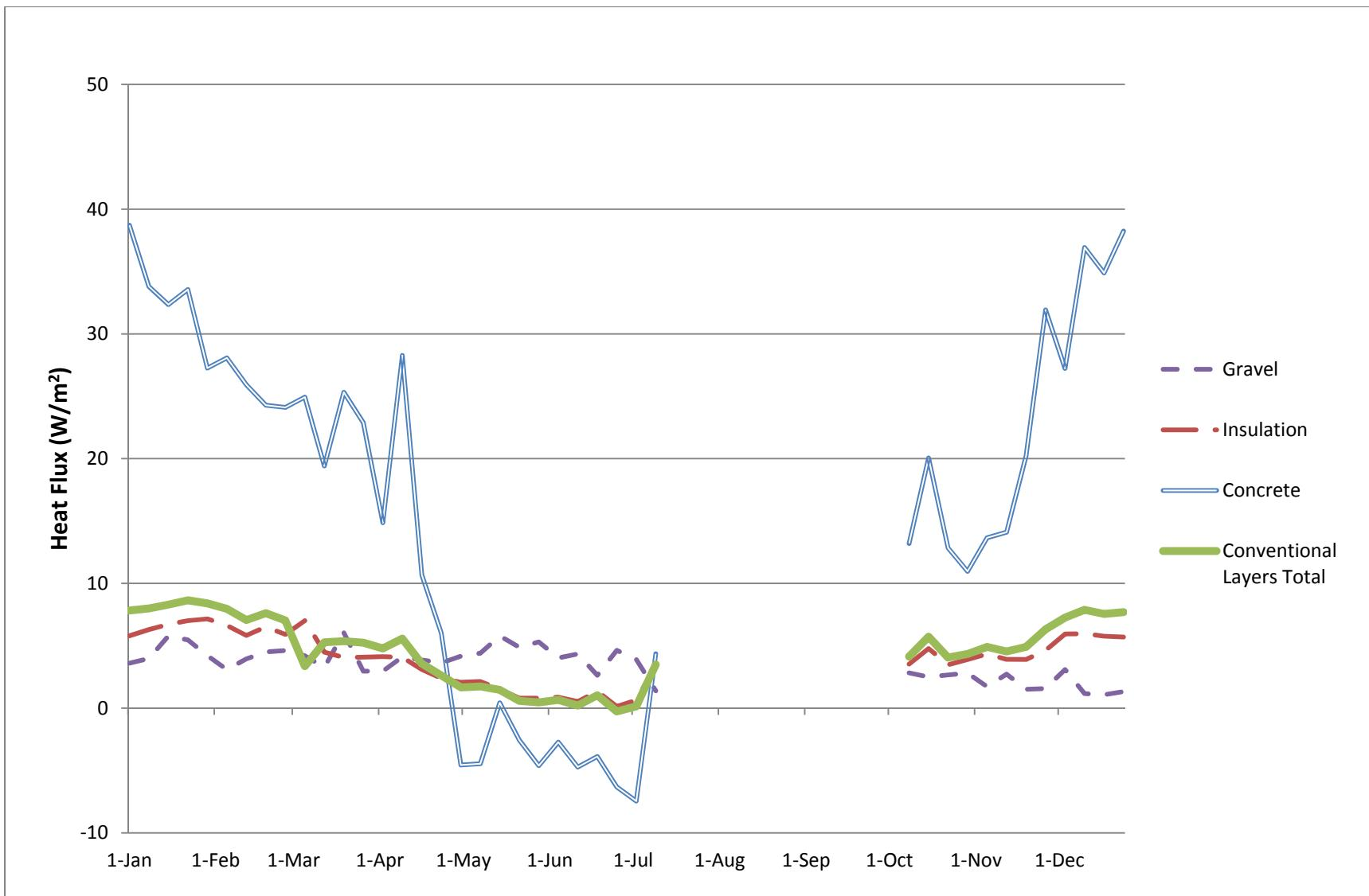
**Figure 2:** Average weekly heat flux through Hamerschlag Hall green roof layers in 2009
