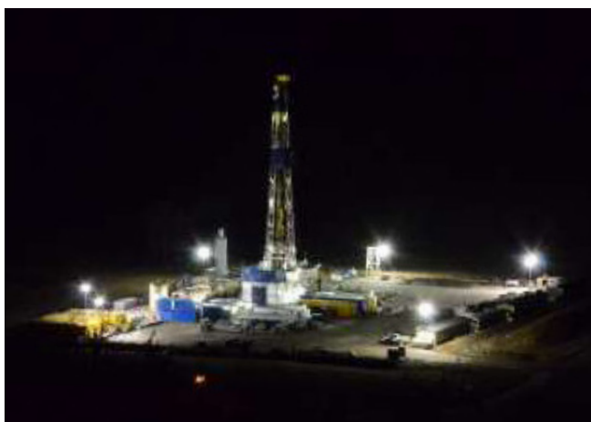
Shale development involves artificial lighting, necessary for security and worker safety, to illuminate work areas at the well pad and near compressor stations. “ Shale Gas Drilling Rig ” by Kelly Maloney, USGS
