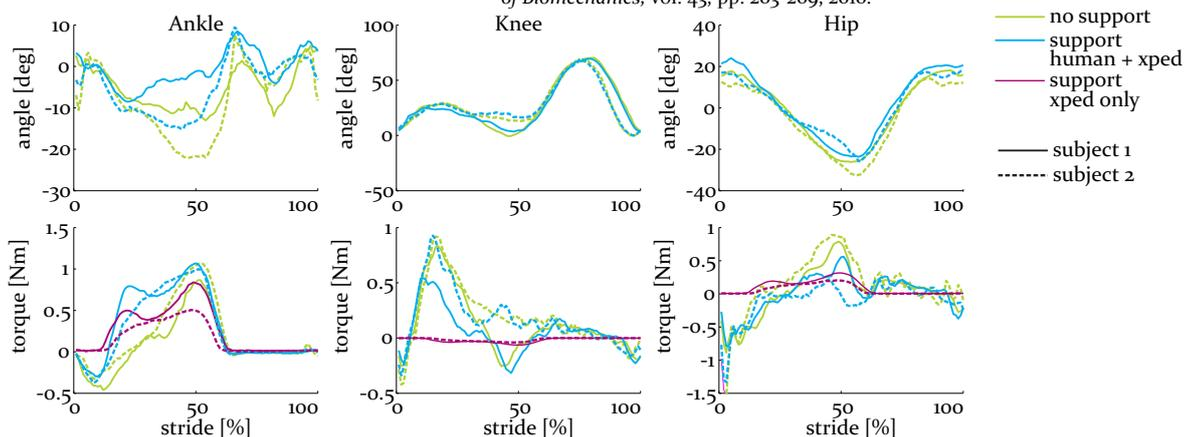
Fig. 2: Test results for walking with the XPED with and without the support of exotendons. Upper row shows joint angles. Bottom row shows joint torques. (Plantar-)flexion is positive.
