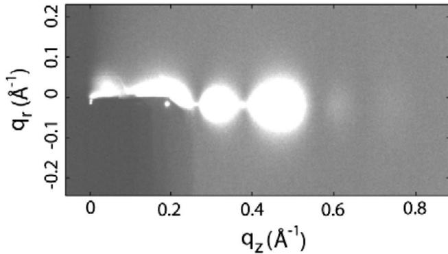
FIG. 1. CCD image of low angle diffuse scattering of DOPC with 30% cholesterol at 30 °C. The dark region  $q_z < 0.2$ ,  $q_r < 0.01$  is blocked by a semitransparent beam stop that attenuates the beam and the very strong first two lamellar peaks.  $K_C$  is related to the  $q_r$  width and  $D_{HH}$  to the  $q_z$  distribution of intensity [7,10].
