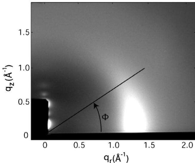
FIG. 2. CCD image of wide angle scattering of DOPC with 30% cholesterol at 30 °C. The beam stop blocks the first five lamellar orders at  $q_r = 0$ .  $S_{xray}$  decreases as the width of the intensity distribution increases in the  $\phi$  direction [11].
