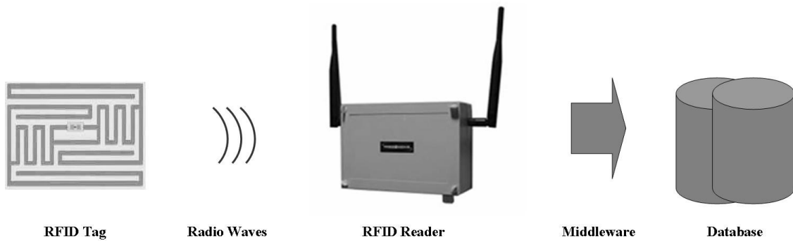
Figure 1: The basic elements of RFID technology are tags, readers, and middleware.
