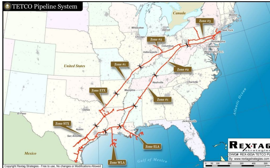
Figure 4.4: The TETCO pipeline system.
