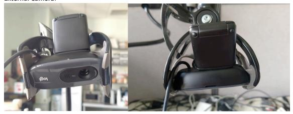
4. Adjust the arm of the mount to point the camera as needed. The mount arms can be difficult to move. We recommend you put one hand on the base of the mount while you move it into place with your other hand. You can point it at a piece of paper on a desk or a physical whiteboard. Manipulating the mount may be easier with two people as they are sturdy.
