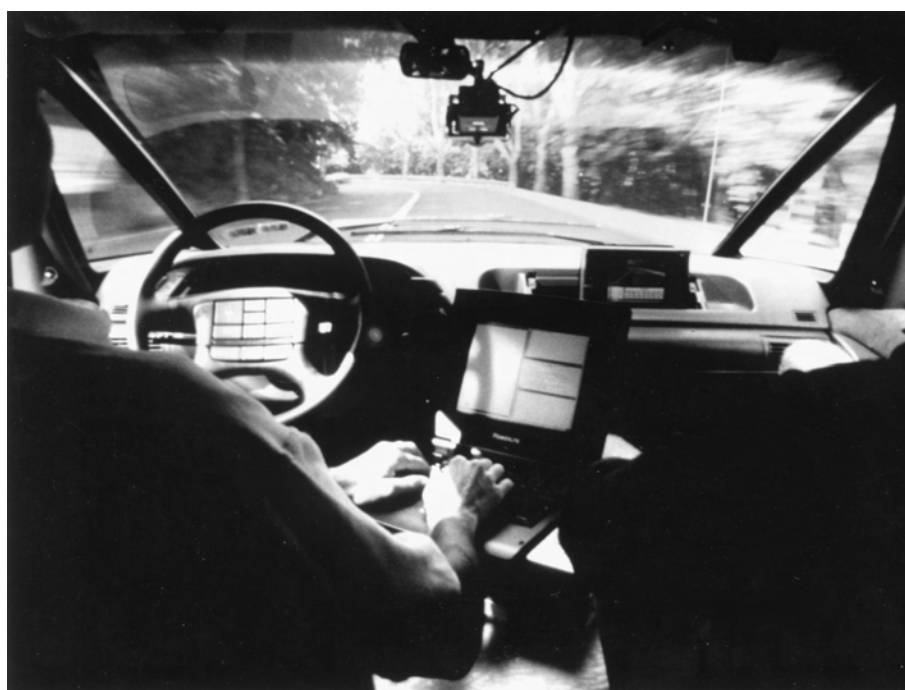
THIS YEAR’S CLASS OF INDUCTEES INTO THE ROBOT HALL OF FAME INCLUDES CARNEGIE MELLON’S OWN NAVLAB 5, A MODIFIED 1990 PONTIAC MINIVAN THAT DID 98 PERCENT OF THE STEERING ON A TRIP ACROSS THE U.S.
