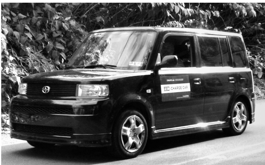
THE CHARGE CAR TEAM USED SMART POWER MANAGEMENT ARCHITECTURE TO CONVERT A 2001 SCION xB FROM GAS TO ELECTRIC.
