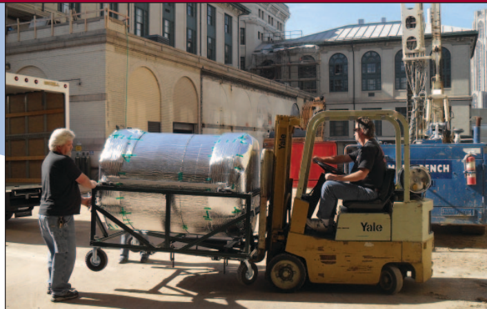
Top: Amy Woodhall (behind the CDC), Gary Wilkin and postdoctoral associate Naomi Jarvis inspect the insulation and bubble wrap around the CDC prior to loading it on the transport van. The wheeled cart was specially designed with shock absorbers and the air pressure in the tires was lowered during transport to Jefferson Lab.
