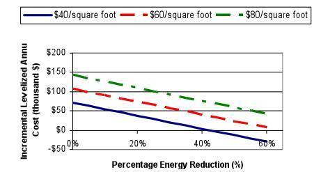
Figure 5.4.1 – Sensitivity analysis for CFA window replacement costs
