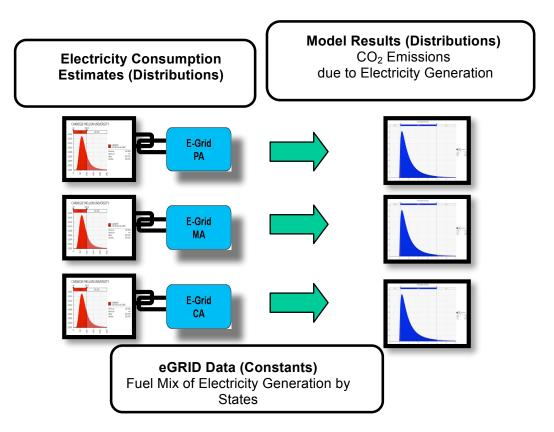
Figure 7.5.5 – Method used to convert electricity use into CO<sub>2</sub> emissions for each school
