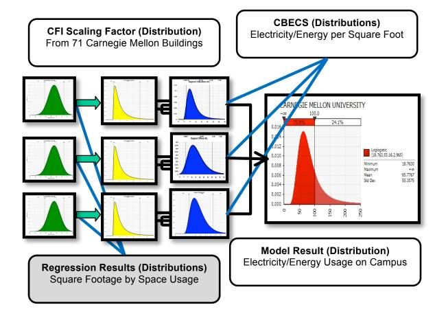
Figure 7.4.5 – Overall method of estimating electricity use for schools in CFI database
