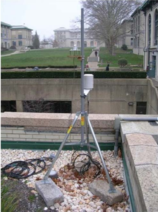
Figure 3.3 Tripod with Tipping Bucket Rain Gauge on the Hamerschlag Hall green roof (Anumol et al., 2010).
