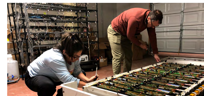
CMU EPP and Materials Science and Engineering PhD student Katrina Ramirez-Meyers and Trustee Professor in Energy Jay Whitacre work on a used hybrid bus battery pack utilized in an Energy Science, Technology and Policy Project Course.
