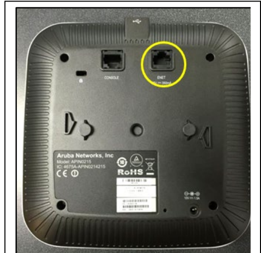
Back of Aruba model AP-215 (similar to 214, 314, and 315) showing “ENET” port in upper right (circled in yellow).
