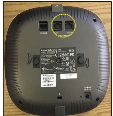
Portal side of AP-324 and AP-325, showing “ENET0” and “ENET1” ports (circled in yellow).
