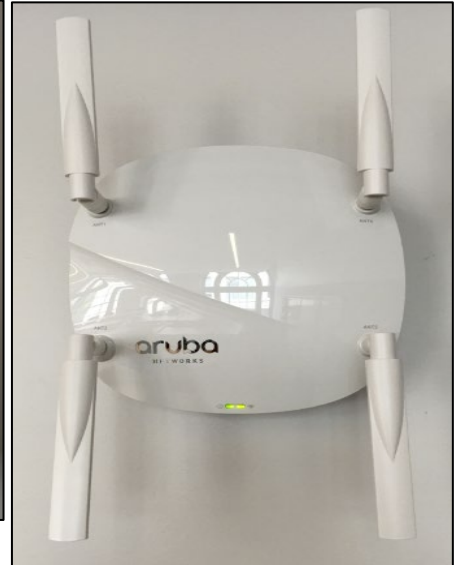
Aruba 324 with antenna using a 900 series box mounted on solid surface
